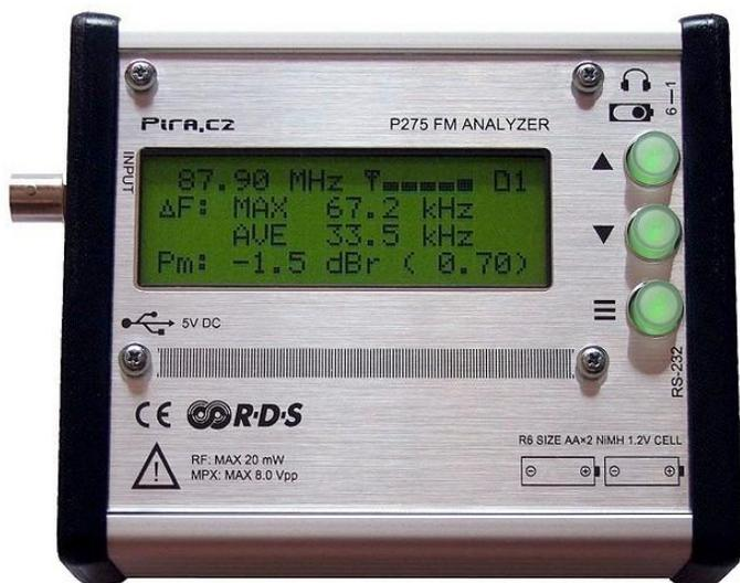
The P275 analyzer is an essential piece of equipment for all FM radio stations to ensure the best audio quality and compliance with basic technical broadcast standards. It may be used for fixed installation as well as for daily work in the field. Durability and RF immunity is assured by the laser machined aluminium case with internal steel frame. The front panel is protected by an acrylic layer.
